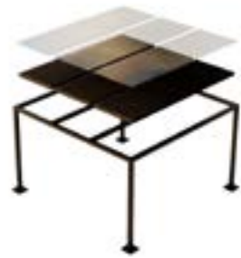
Aluminium strip ceiling + Glass Thickness: 20 + 8 mm Type 01 5x5 m Type 02 6x5 m Type 03 4x4 m
