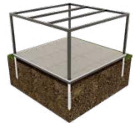
Type C Floor & Screw - 170 mm above the ground Pile depth: 1490 mm
